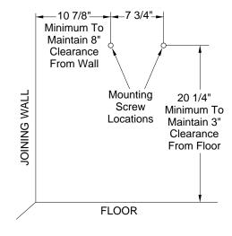
Figure 5 - Mounting Screw Locations
